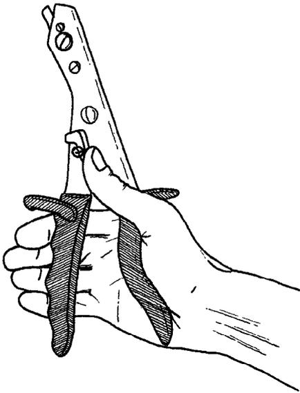
Figure 6. Shanks with notches for the fingers, which do not suit the user.
